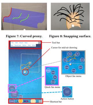
Figure 9: The user interface of *Mobi3DSketch*. The functions of the action button change with the selected tools.
