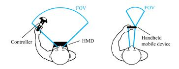
Figure 2: Small-sized mobile screens result in a much narrower field of view (FOV) than VR HMDs. 2D/3D input and display are coupled in our case.
