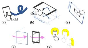
Figure 6: Representative operations in our multimodal interface for mobile 3D sketching. (a) Mid-air 3D drawing, (b) surface-based 2D drawing, (c) proxy creation, (d) proxy rotation, and (e) cloning.
